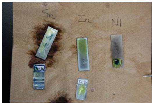
Fig. 11 Corrosion protection of plated iron
